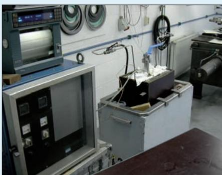
Typical set-up for testing a small valve.
