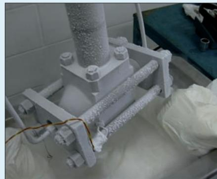
The rate at which a valve is cooled can be varied according to the needs of the client.
